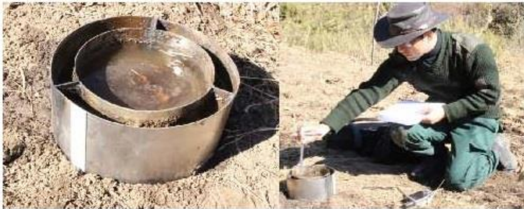
Figure 6: (Left) Improvised double ring infiltrometer, (Right) taking note
