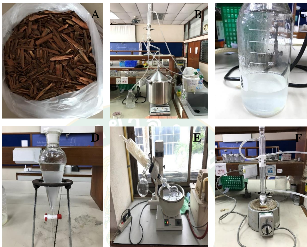
Appendix figure 2 Chemical Compound Isolation: A. Sample cinnamon bark; B. Simple hydrodistillation setup; C. Distillate product containing cinnamaldehyde; D. Separation of Cinnamaldehyde; E. Rotary evaporation of excess solvent; F. Reflux set up
