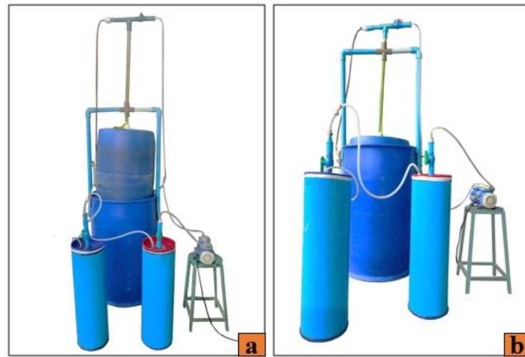
Figure 3.12 Experimental set-up for biogas purification: (a) before experiment; (b) after experiment
