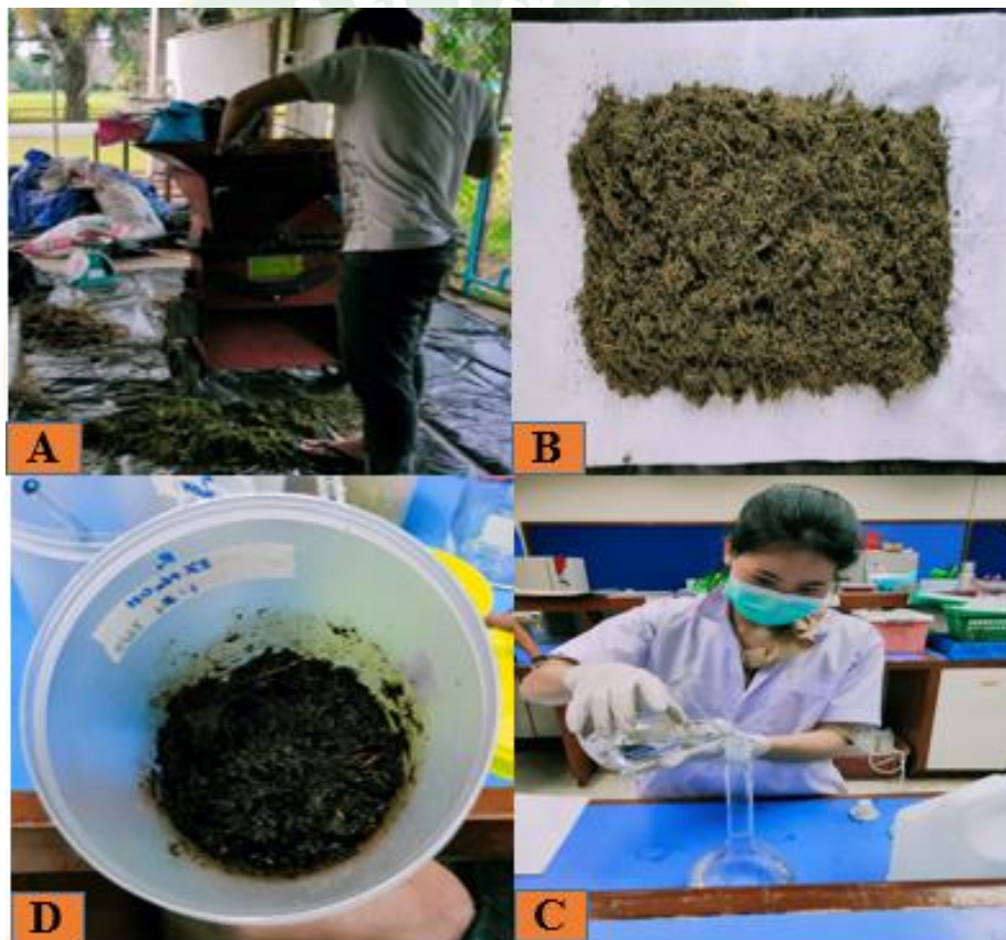
Figure 3.4 Alkaline pretreatment of water primrose (fresh) (A) Shredding material; (B) Sample preparation; (C) Alkaline solution preparation; (D) Pretreated sample
