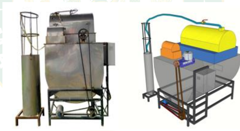
Figure 3.10 Anaerobic digestion system of big scale
