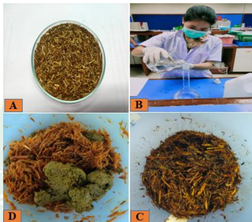
Figure 3.6 Co-digestion of water primrose and cow dung (A) Sample preparation; (B) Alkaline solution preparation; (C) Pretreated sample; (D) Sample mixing
