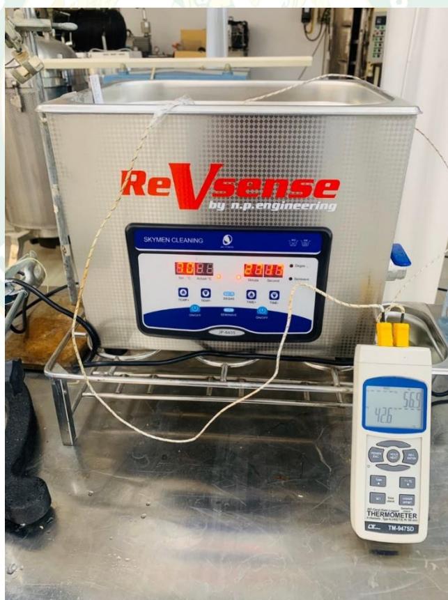
Figure 31 Heating and ultrasonic treatment at 100 Watt power, frequency 40 kHz
