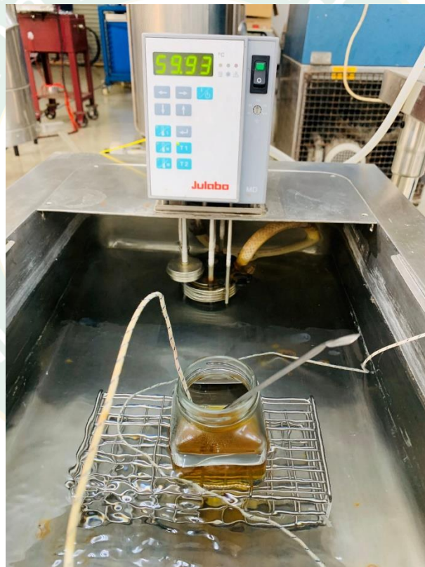
Figure 29 Heating honey by heating bath
