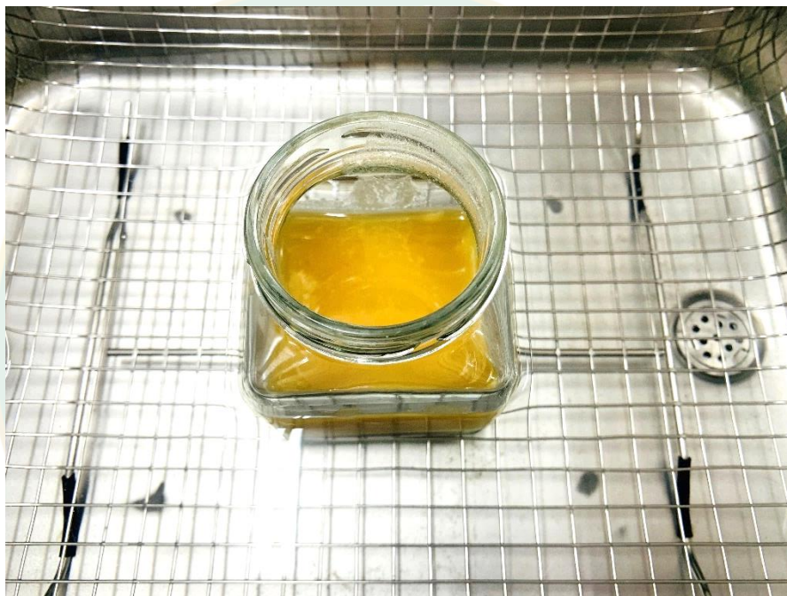
Figure 45 the mixed honey was treated with ultrasonic at 40 kHz and 0.15 \text{ Watt/m}^2 in chilled water
