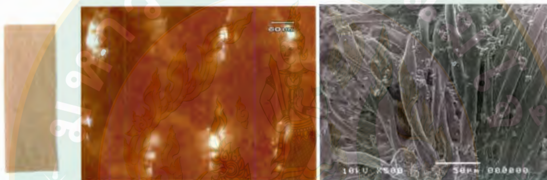
Figure 45 Optical microscope and SEM images of cotton fabrics finished with guava leaf extract
