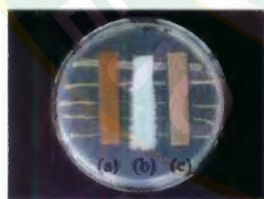
Fig. 6. Antibacterial activity results against S.aureus of (a) cotton fabric finished with guava leaf extract; (b) unfinished cotton fabric; (c) cotton fabric finished with MCs containing guava leaf extract.
