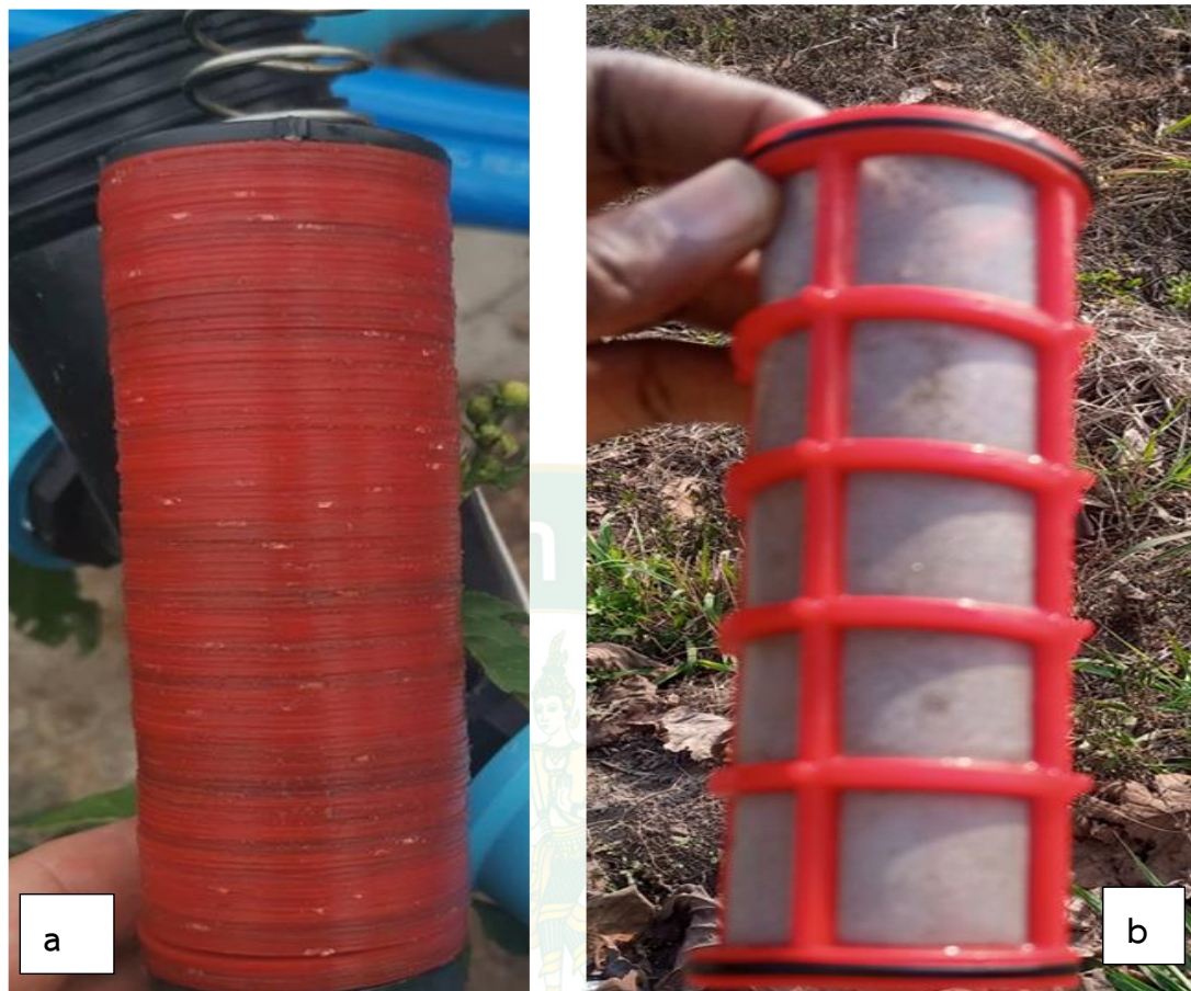
Figure 22 Disc filter and mesh filter.
